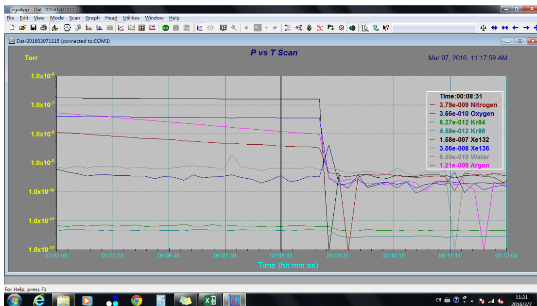
Fig. 7: Data recorded during a measurement. The acquisition continues after closing V4 (no more flow to the RGA), to check that the vacuum is restored, so presumably the background remained the same during the measurement.
