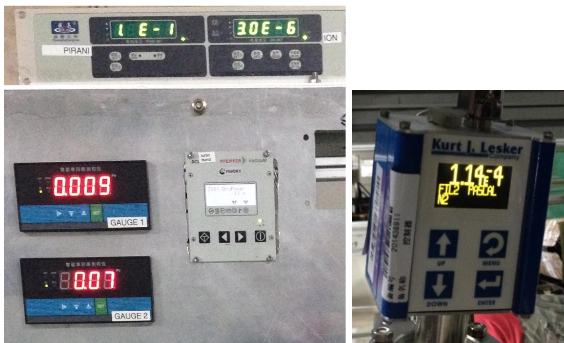
Fig. 2: Left: main displays of the front panel, with their normal reading when the system is under a good vacuum. Gauge 1 is the high P (range up to 10 bar) gauge of the bus, Gauge 2 is the front piping gauge with same range. Both displays are in bar. The controller in the top displays on the left the pressure (in Pa) of the Pirani gauge of the bus (range 0.1-1e5 Pa), which in these conditions is normally below range, and on the right the pressure (in Pa) of the ion gauge on the RGA side (range to 10 Pa). Never turn this gauge on if you think the pressure could be above 5-10 Pa. Right: Lesker ion gauge, placed in the back of the front panel. It measures the bus pressure (in Pa) when it is under high vacuum. Its range is up to 6.7 Pa. Never turn this gauge on if you think the pressure could be above 3-6.5 Pa (yes, the Lesker gauge takes less pressure than the RGA side ion gauge).
